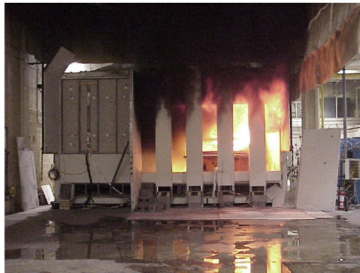
Figure 4-6. Multiple workstation fire experiment.
